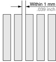
2) Coil terminals (Terminal No. 1 & 2) polarity should be arranged in the same direction.
