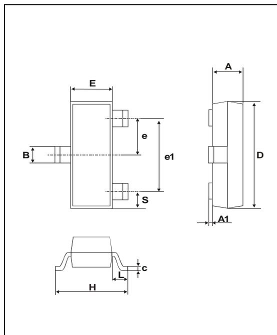
Figure 8. Footprint (dimensions in mm)
