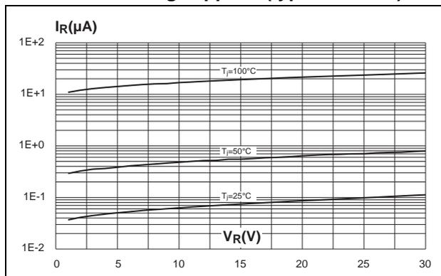
Figure 4. Reverse leakage current versus junction temperature
