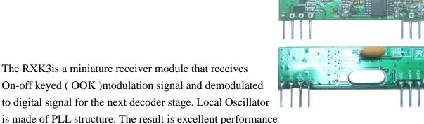
to digital signal for the next decoder stage. Local Oscillator is made of PLL structure. The result is excellent performance in a simple-to-use ,with a low external component count. The RXK3 is designed specifically for remote-control and wireless security receiver operating at 315/395/434MHz in the USA under FCC Part 15 regulation.
