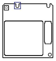
You can insert machine screws through the structure fixing holes and metal fasteners and fasten with nuts to firmly connect the MG301 B2B module to the user interface board [1]. The metal fastener is placed between the MG301 B2B module and user interface
