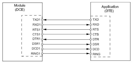
When an MG301 B2B module receives an SM (Short Message), a low-level signal is output through the RING (pin 38) for 1s, as shown in Figure 3-9.
