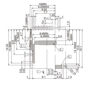
Note 1 > 4 indicates the center line of the microSD card slot.
