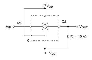
$$R_{ON} = 10 \times \frac{\left(V_{IN} - V_{OUT}\right)}{V_{OUT}} \left[k\Omega\right]$$
