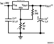
Full output current not available at high input-output voltages †Optional—improves transient response
