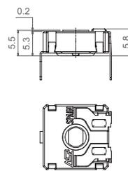
Position indicating notch included on all LV15 rotors, except types M and P.
