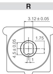
This drawing shows the rotor at 50% position in order to better depict the dimensions and tolerances, it is not a valid delivery option of the 16 position version.
