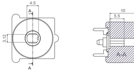
This drawing shows the rotor at 50% position in order to better depict the dimensions and tolerances, it is not a valid delivery option of the 16 position version.
