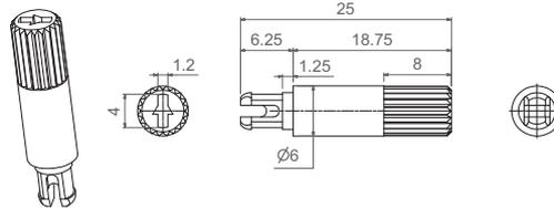
Thumbwheels are available in different colors (color chart in "how to order" section) and with self-extinguishable property according to UL 94 V-0, under request. Thumbwheels can be mounted on the potentiometers at ACP or sold separately. ACP can study special thumbwheel designs.
