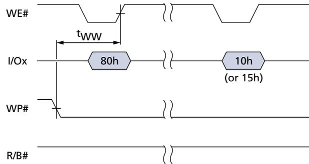
Figure 51: PROGRAM for INTERNAL DATA MOVE Enable
