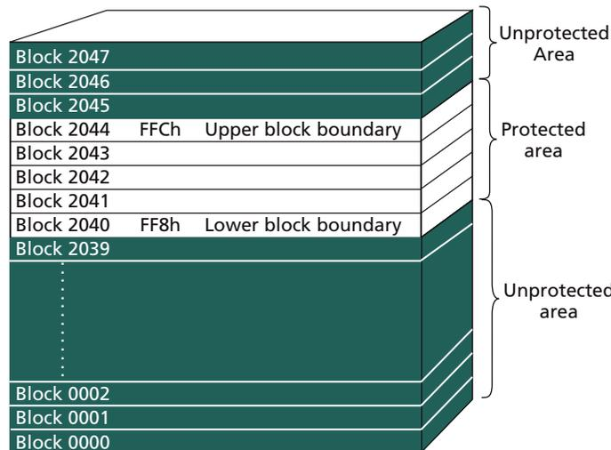
Table 13: Block Lock Address Cycle Assignments
