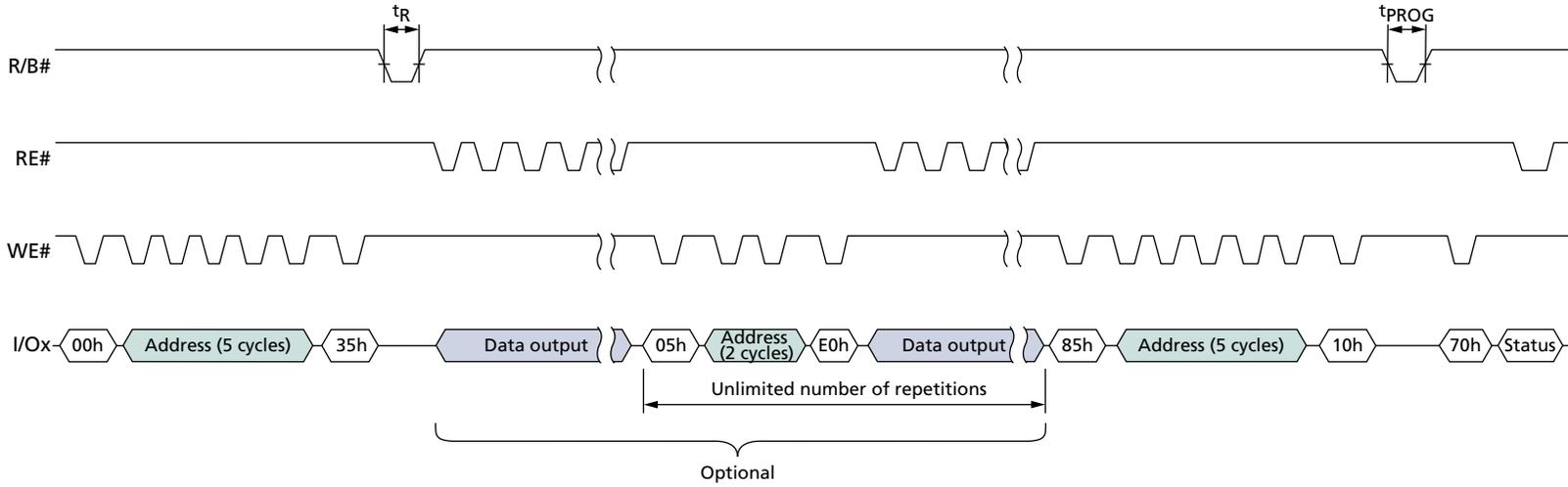
**Figure 29: INTERNAL DATA MOVE with Optional RANDOM DATA Output and RANDOM DATA Input**
