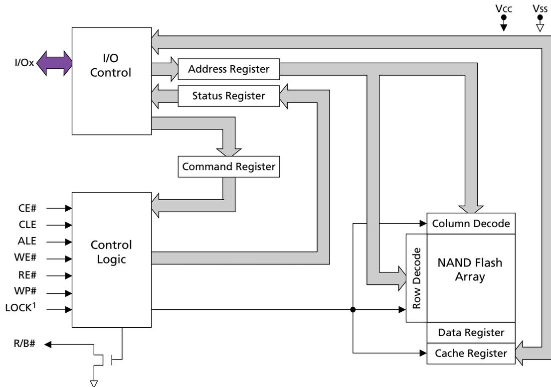
Notes: 1. LOCK pin is used for 1.8V device.
