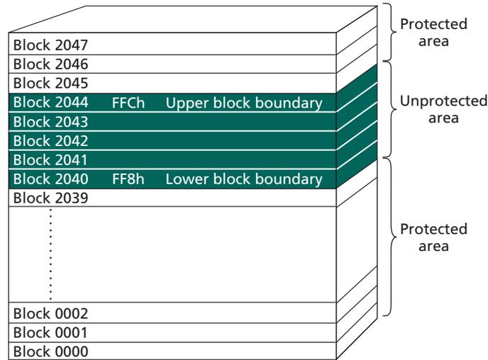
Figure 32: Flash Array Protected: Invert Area Bit = 1
