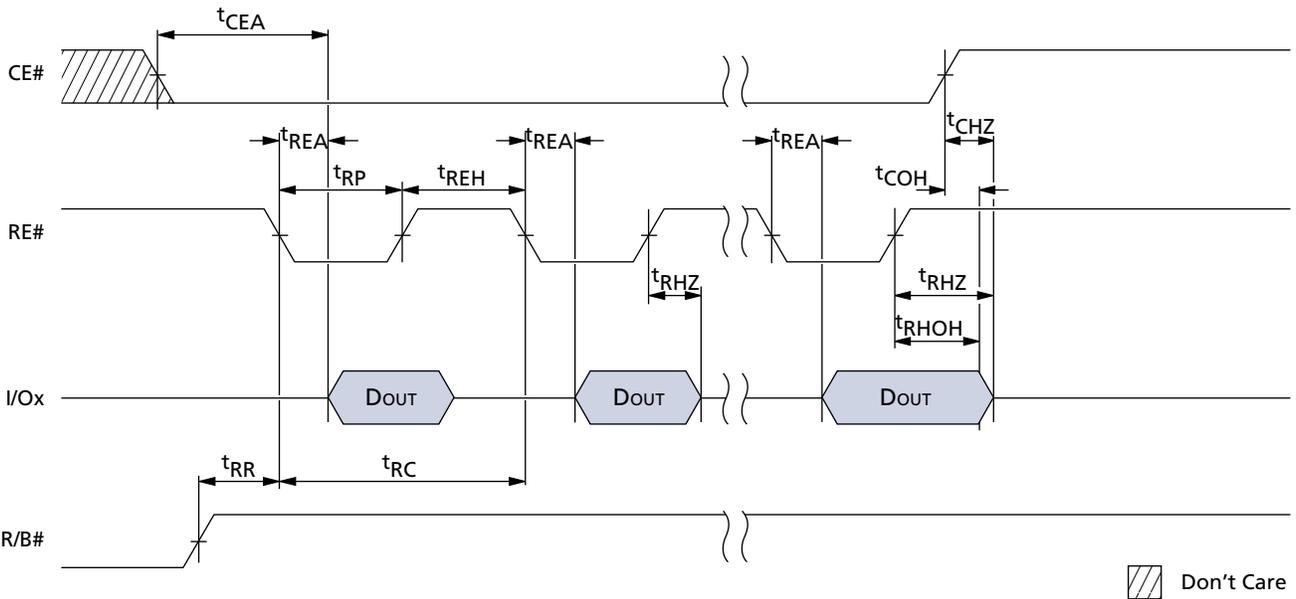
Note: Use this timing diagram for  $t_{RC} \geq 30\text{ns}$ .
