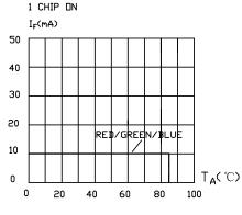
MAXIMUM FORWARD DC CURRENT VS. AMBIENT TEMPERATURE
