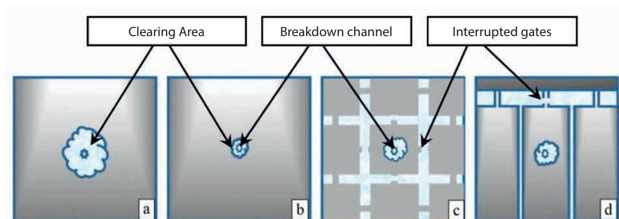
a and b: not segmented metallization;
