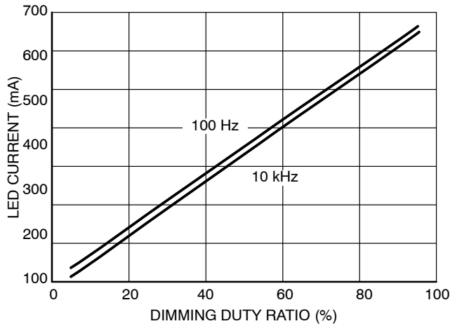
Figure 13. LED Current vs. Dimming Duty Ratio
