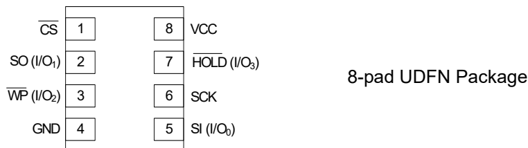
Figure 2-1. Adesto AT25SF128A Flash Memory Package Types
