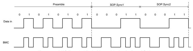
Figure 22. BMC Encoded End of Preamble, Beginning of SOP
