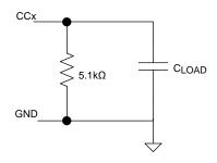
Figure 25. Test Load for BMC Transmitter
