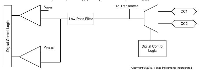
Figure 27. USB PD BMC Receiver Schematic
