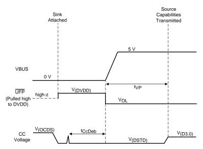
Figure 3. Timing Illustration for  $t_{\text{CcDeb}}$  and  $t_{\text{VP}},$  Under Persistent Fault Condition
