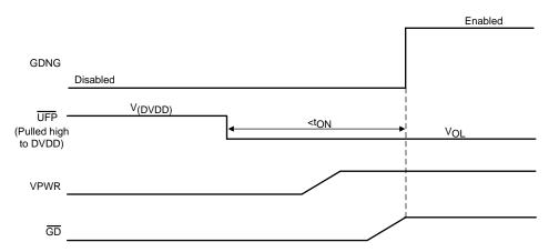
Figure 6. Timing Illustration for ton
