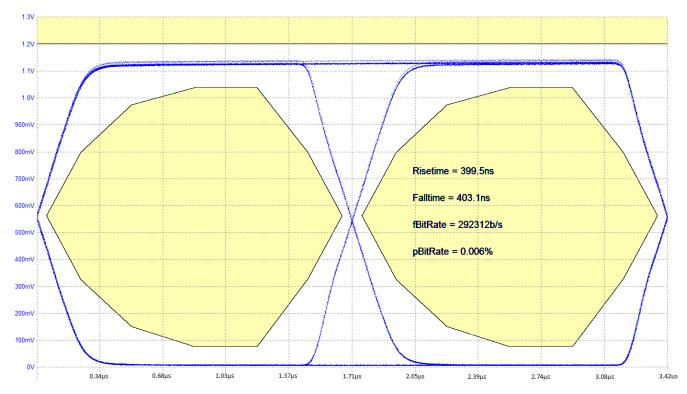
Figure 26. Transmit Eye Diagram (BMC)
