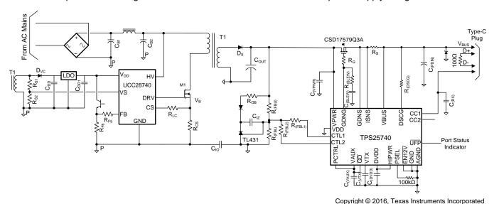
Figure 45. Captive Cable Adapter Provider Conceptual Schematic
