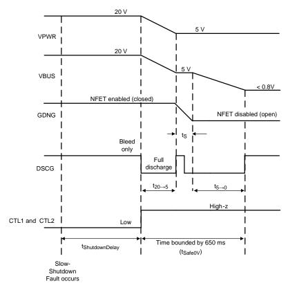
Figure 29. Illustration of Slow-Shutdown VBUS Discharge
