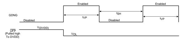
Figure 4. Timing Illustration for t<sub>SH</sub> and t<sub>VP</sub>, with VBUS Shorted to Ground
