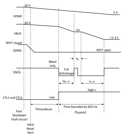
Figure 30. Illustration of Fast-Shutdown Discharge
