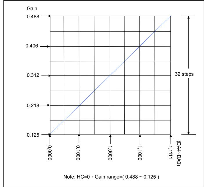
The 6 bits (bit 5~bit 0) of the configuration register set the gain of output current, i.e., G. As total 6-bit in number, i.e., ranged from 6'b000000 to 6'b111111, these bits allow the user to set the output current gain up to 64 levels. These bits can be further defined inside configuration register as follows:
