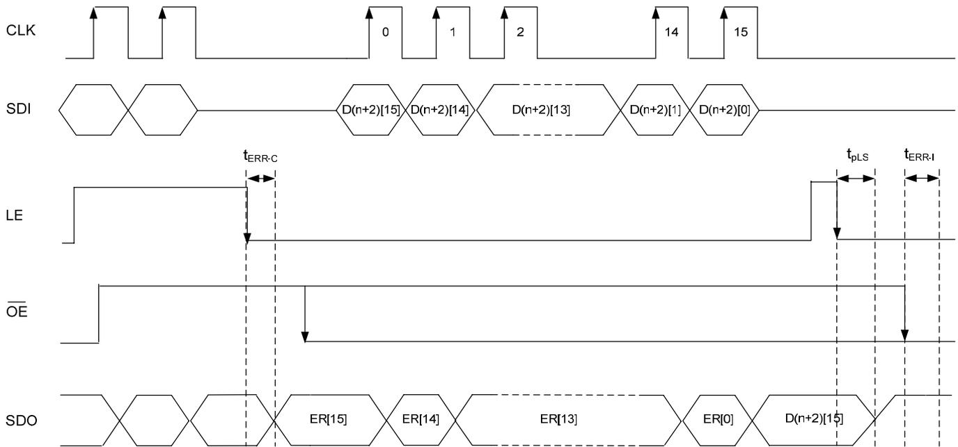
1. Conditions required to activate the short-circuit detection: (1) falling edge of LE and (2)  $\overline{OE}$  =High
