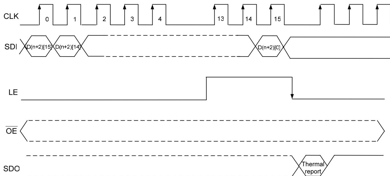
At the falling edge of LE, if the driver is overheated, the code "7FFF(HEX)" is delivered to SDO; otherwise, the code "FFFF(HEX)" is latched to shift register.
