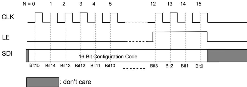
After entering the writing configuration mode, the system controller sends a 16-bit configuration register to 16-bit shift register through the SDI pin. Then the falling edge of LE will transfer the contents in the shift register to a 16-bit configuration register rather than the 16-bit output latch.
