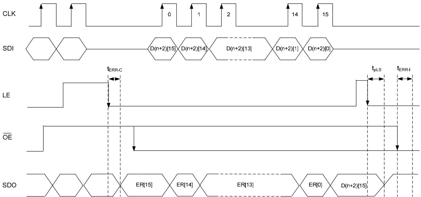
1. Conditions required to activate the open-circuit detection: (1) falling edge of LE and (2)  $\overline{OE} = \text{High}$
