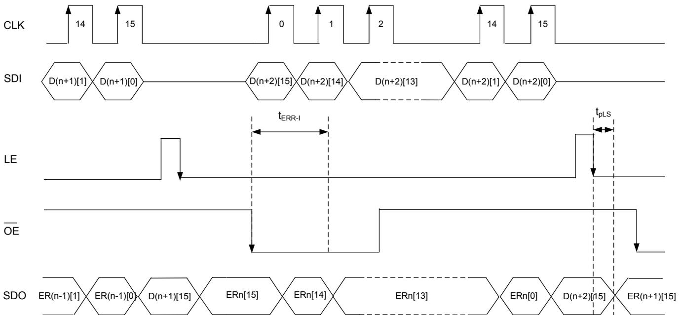
1. Condition of valid error detection: (1) Data = "1" (2)  $\overline{OE}$  (low) >  $t_{ERR-I}$
